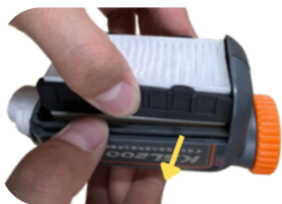
Step 4: While holding the Inner Case and the rubber frame, pull open the outer case.
