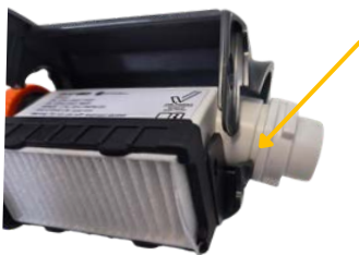
Step 7: Place the filter assembly back in the Inner Case, making sure the Inner Case edge aligns with the groove at the outlet of the Main Filter.
